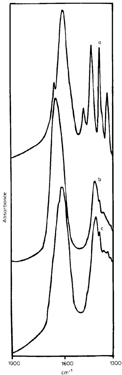
Fig. 1. Fourier transform-infrared spectra of D-glucuronate anion and its platinum-ammine complexes in the range 1900–1300 \text{cm}^{-1} for: (a) sodium D-glucuronate \cdot 2\text{H}_2\text{O} ; (b) cis -[Pt(D-glucuronate)( \text{NH}_3 ) _2 ](D-glucuronate) \cdot \text{H}_2\text{O} ; (c) trans -[Pt(D-glucuronate) _2 ( \text{NH}_3 ) _2 ] \cdot \text{H}_2\text{O} .
